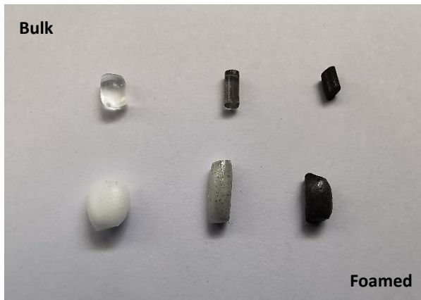
Figure 1a: Bulk and foamed TPU/Gr granules (from left to right: Pure TPU, TPU/0.1%Gr, TPU/1%Gr).
